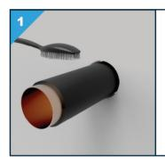
Make sure that the service penetration and the gap are free from dust, dirt and grease. Moisten the structure, if necessary.
